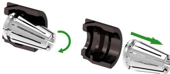
4. Tilt collet up to the marking until it is removed from the eccentric ring. Remove collet.
