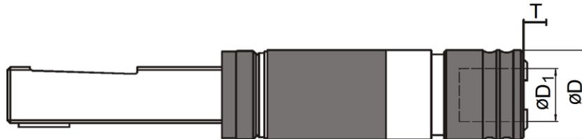
Picture 2: Dimensions of the quick-change tap holders SFM-L-Z
